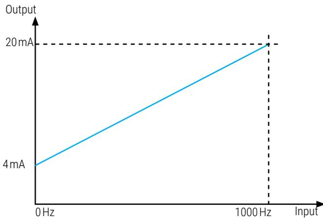
Selecting the predefined code '025' configures a range of 0/1000 Hz=4/20 mA, and the values configured are as indicated below:
