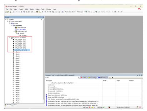
Double-click the corresponding module to view the corresponding I/O address and set the corresponding mapping relation.
