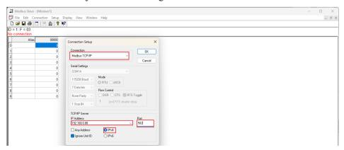
Right-click on the blank space of the Mbslave1 window - select 'Slave Definition', and set as follows in the pop-up window. The specific parameters should correspond to the channel parameters set by the 'Modbus TCP Slave device' in CODESYS. If the parameters do not correspond, it may cause errors and Communication exception:
