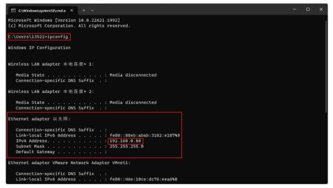
It can be seen that the IPv4 address used here is 192.168.0.88, so the IP address of the slave station it should enter in the CODESYS interface is 192.168.0.88, and the port can be consistent with the port set by the third-party slave station. The setting here is 502.
