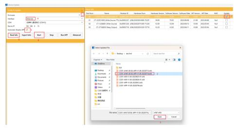
The above is the firmware upgrade process. Similarly, it can use this method to upgrade the equipped I/O module.
