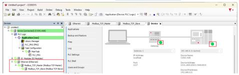
All devices are in the running state, indicating that the connection is successful. Now click on the 'ModbusTCPSlaveI/O Mapping' menu of the 'Modbus TCP Slave Device' to monitor the current value of the channel mapping:
