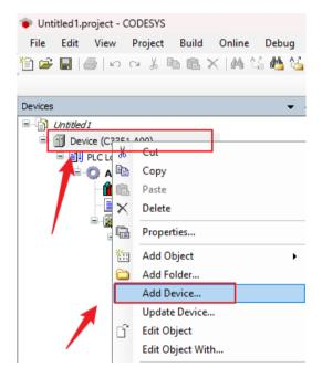
Add an 'IO Modules device' to the project in the pop-up interface. If this device is not found, refer to 5.2.1 to create a project and install device description file.
