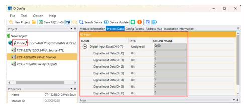
Note: For digital input modules, it could right-click the module and manually add a 'counting sub-module'. After the addition is complete, the configuration must be downloaded again.
