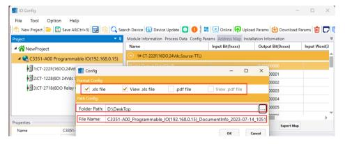
The example of the generated file is as follows, and a total of 5 aspects of information are generated, including the overview of the submodules, the statistics of the number of submodules, the schematic diagram of the submodules, the address table, and the parameter settings of the submodules:
