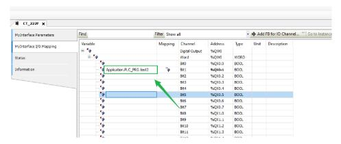
It could make a simple output variable assignment program, and observe the changes of the indicator lights of the C3351 physical equipment. Connect QX0.0 and QX0.1 of BT-221F to the variables test1 and test2 in two ways. The first way is the way marked in green in the above picture, and the second way is the way marked in red in the picture above. Two ways can associate channels with variables.
