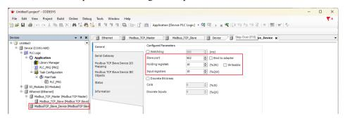
After the setting is complete, we click the option of 'ModbusTCPSlaveDeviceI/O Mapping' to view the address mapped in the C3351 device by the newly established slave device.
