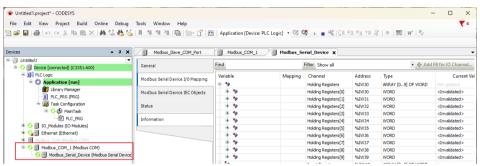
The following is the verification of the communication. The first step is to double-click to modify the input register preparation value to 1111 in the 'ModbusSerialDeviceI/O Mapping' of the 'Modbus Serial Device device', and press 'Ctrl+F7' to write:
