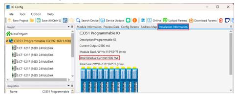
It could click a single I/O module icon to pop up the hardware information of the corresponding module.
