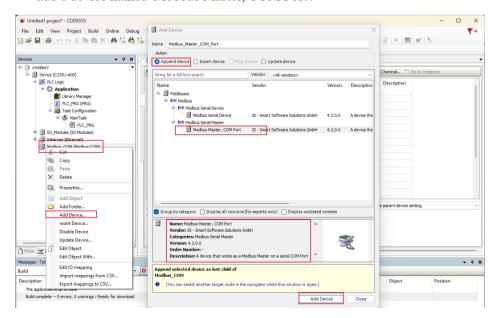
Right-click the 'Modbus Master, COM Port device' just created in the project tree, select 'Add Device' → add a device named 'Modbus Slave, COM Port'.
