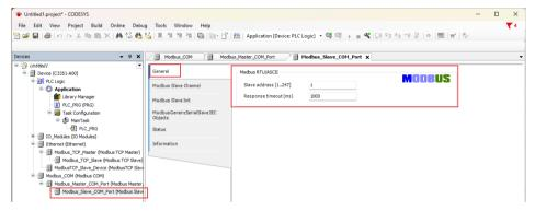
Then select 'Modbus Slave Channel' - 'New Channel', and set various parameters in the pop-up window:
