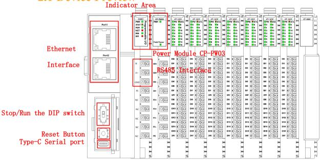
Reset Button: press and hold for 5s so it could to reset the C3351 to its initial state, including device configuration parameters, user program storage area, power-down storage area, etc. will be cleared or reset.
