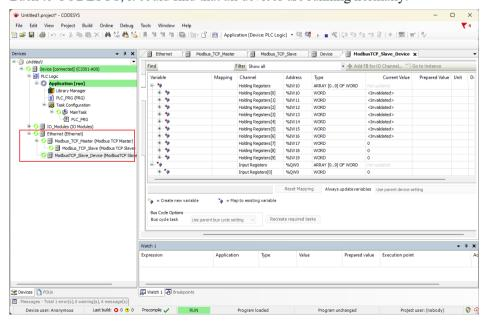
The following is the verification of the communication. The first step is to double-click to modify the input register Prepared Value to 1111 in the 'Modbus TCPS lave Device I/O Mapping' of the 'Modbus TCP Slave Device', and press 'Ctrl+F7' to write:
