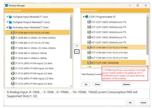
In this example, it is indicated that the power module should be inserted into slot 11. After the power module is added, the total remaining current displayed on the lower side of the selected module will change to a black font, and other I/O modules can be added behind it.
