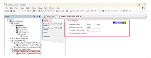
Next, double-click 'Modbus Slave COM Port Device' → select 'General' on the main interface on the right, and set the slave station address and response timeout time:
