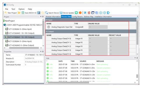
Configured parameter: The module parameter information can be showed and modified, such as IO adapter module, PLC and I/O modules
