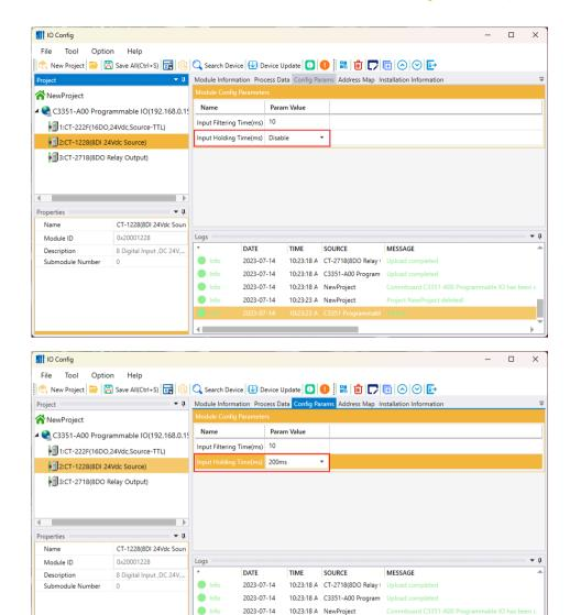
After the setting is complete, right click on the C3351 device in the project directory bar → 'Download Params'. It can realize the modification of configuration parameters of C3351 equipment and I/O modules.
