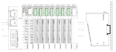
After the module is installed vertically, press the lock on the top of the module to ensure that the module is installed in place, and the distance between the module and the upper and lower contact surfaces of the 35mm Din rail is less than 1mm. Press the lock on the left side of the C3351 device counterclockwise to lock the Din rail.
