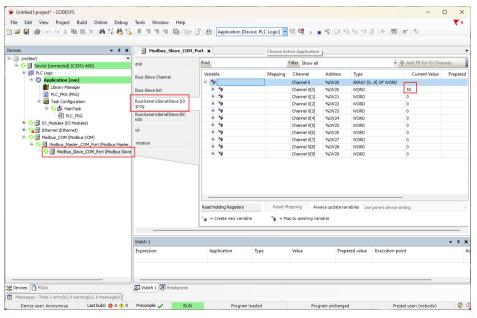
So far, the Modbus RTU master function test of the C3351 device is completed.
