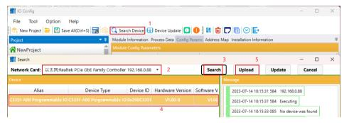
The software will automatically create the project, as shown in the figure below.
