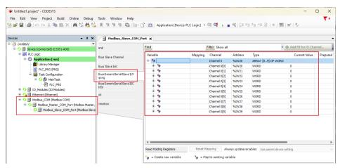
Go back to the third-party slave station simulation software 'Modbus Slave', double-click the first data, and a modification window will pop up, then modify the value of the first data to 55:
