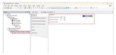
Similarly, double-click the 'Modbus TCP Slave device' in the CODESYS interface - select the general settings of Modbus TCP's 'slave station IP address', 'response timeout' time and 'port number' in the main interface on the right. This IP address is the IP address of the third-party slave station simulation software, that is, the IP address set by the local PC, press the Win+R key, enter CMD and press Enter:
