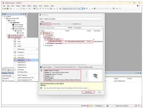
Similarly, right-click the 'Modbus TCP Master Device' just added to the project → 'Add Device' → add a device named 'Modbus TCP Slave', the supplier is 3S – Smart Software Solutions GmbH.
