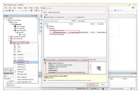
Next, it could set the parameters of the slave station and the third-party master station. Here, the third-party master station simulation software Modbus Poll is used to simulate the connection of the slave station device. Similarly, double-click the Modbus COM 1 device just added to the project → select 'General' option and configure the serial port.
