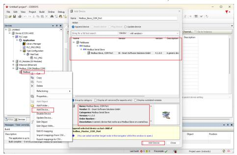
The required equipment has been created. Next, we configure the parameters of the master station and the third-party slave station simulation software Modbus Slave. Double-click the 'Modbus COM device' in the project tree-select 'General' in the main interface on the right, and then configure the serial port according to the actual situation:
