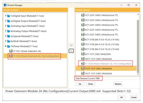
When actually installing the module, it needs to add a power module (CT-7220) to slot 11. The CT-7220 power module does not require configuration and does not occupy any slot. So, it is grayed out in the screenshot.
