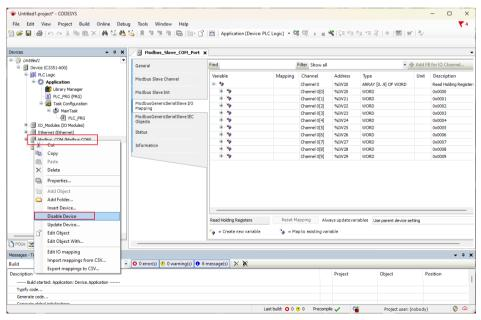
Right-click the newly created Modbus COM 1 in the project tree, select Add Device → add a device named 'Modbus Serial Device'.
