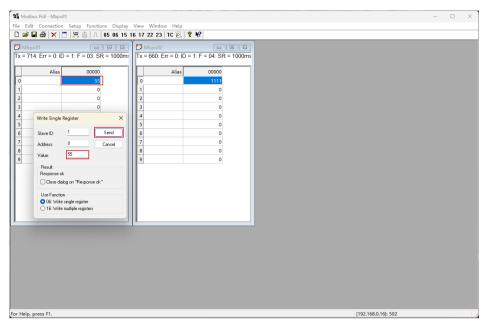
Back to the CODESYS software, it could find that the first WORD value of the holding register has been changed to 55, indicating that the communication function is normal:
