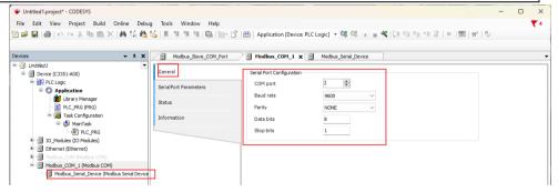
Double-click 'Modbus Serial Device', and select 'General' in the main interface on the right, and set the unit ID, holding register length, and input register length in the configuration parameters:
