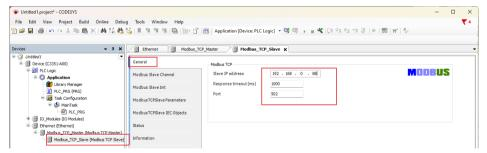
Next, continue to set the Modbus slave station channel of the "Modbus TCP Slave device" → the step "Add Channel" as shown in the figure below, here a channel type of "Read Holding Registers" is added, and its length is 10 WORD:
