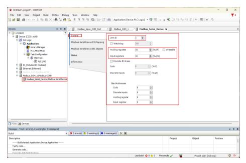
After the setting is complete, we click the option of 'Modbus Serial Device I/O Mapping' to view the address mapped in the C3351 device by the newly established slave device.
