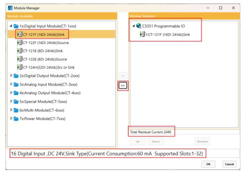
The power consumption of the selected I/O module will be displayed in the lower left corner. After configuration to the rear side, the total remaining current will be displayed on the lower right side. When the current is exhausted, the font will be displayed in red. At this time, a power module needs to be added.
