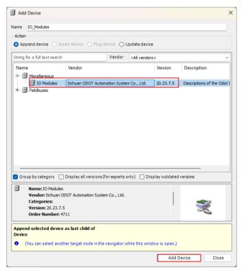
Then select the 'empty' slot, right-click and select 'Insert Device', and insert the required module. For the function of the module, refer to the 1. 7Selection
