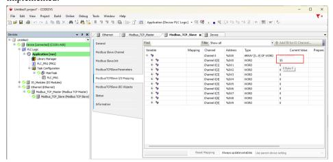
When C3351 is regarded as a server, on the previous basis, right-click 'Ethernet Device' in the project → 'Add Device' → add a device named 'Modbus TCP Slave Device', the supplier is 3S – Smart Software Solutions GmbH.
