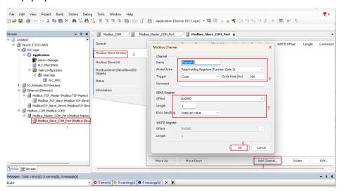
After the addition is complete, we can find that there is an option of 'ModbusGenericSerialSlaveI/O Mapping' in the menu. Click this option to view the address mapped in the C3351 device by the channel just established.
