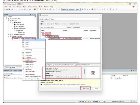
Next, let's set the parameters of the master station and the third-party slave station. Here, the third-party simulation software Modbus Slave is used to simulate the connection of the slave station device:
