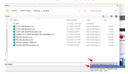
Select (multiple choice) the xml file provided by our company (including C3351 device and IO module) and open it
