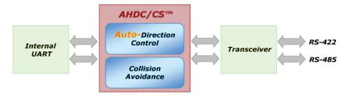
Auto Hardware Direction Control (AHDC<sup>™</sup>) technology makes it easier to manage 2-wire RS-485 half-duplex communications, eliminating the need for software interference. User does not necessary to write extra code for Windows applications to control the half-duplex protocol. Auto Hardware Direction Control (AHDC<sup>™</sup>) technology is the key feature of SUNIX UART, and this function is default enabling.
