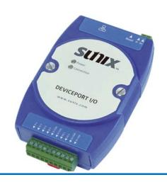
SUNIX EZR5002 utilizes SUNIX EAZInet networking technology to quickly expand two digital input and four digital output signals via Ethernet, allowing users to conveniently implement automation, swiftly incorporate the Internet of Things into their businesses, and raise their competitiveness.
