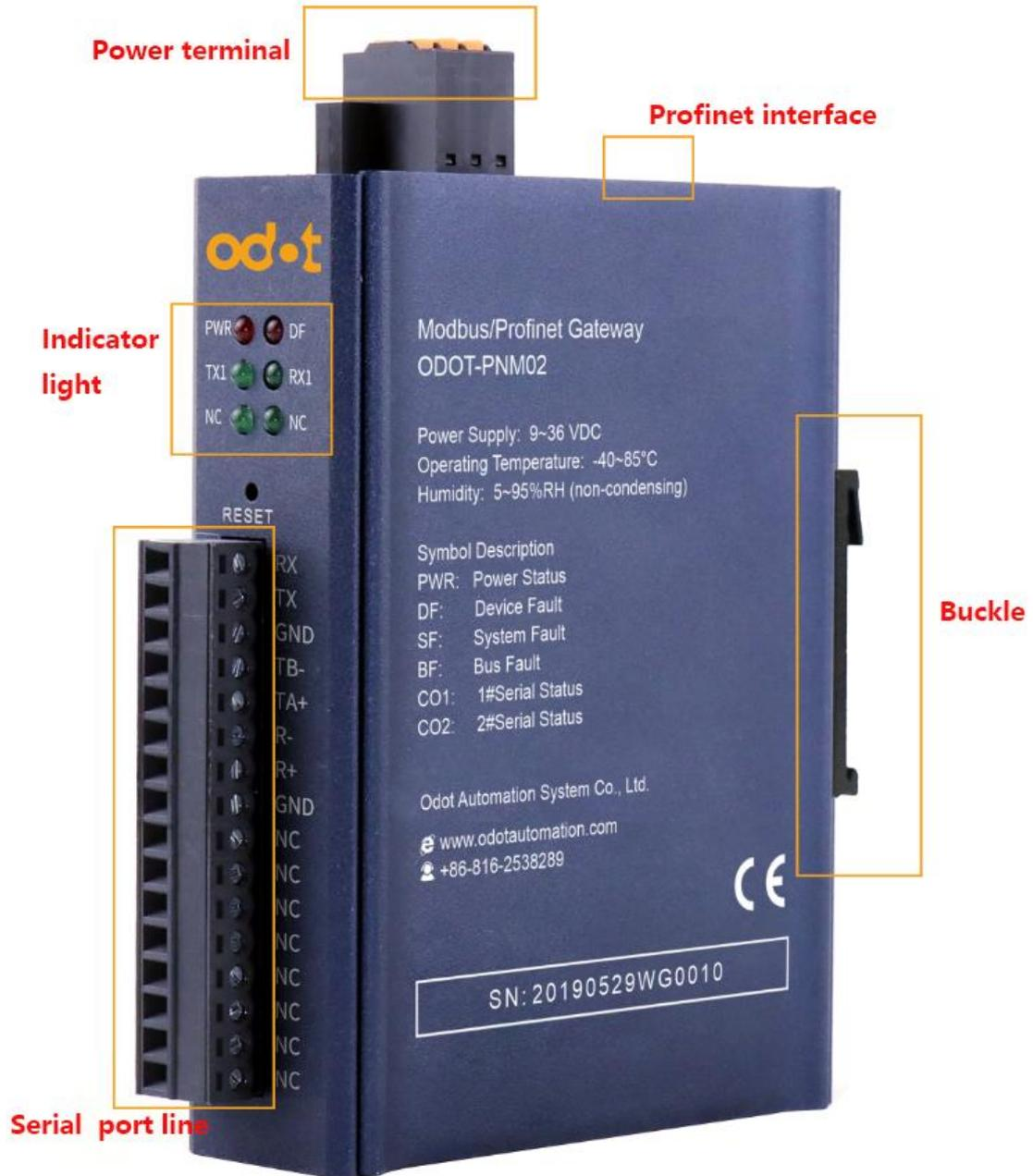
The upper panel has two ProfiNet interfaces and power connection terminals. PORT1 and PORT2, the two interfaces have the same function. These two interfaces have the switch function, that is, the host computer can access the equipment connected to PORT2 through the PORT1
